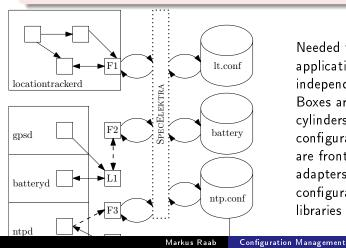
Needed to keep applications independently. Boxes are applications, cylinders are configuration files, F? are frontends or frontend adapters, L? are configuration libraries [7].
